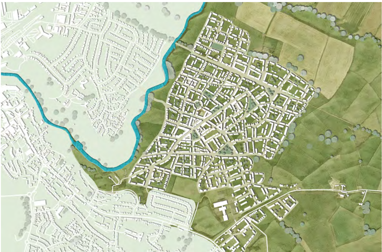
The alternative denser masterplan extends Chippenham to the East, reducing land take from 350 hectares to 120 hectares
