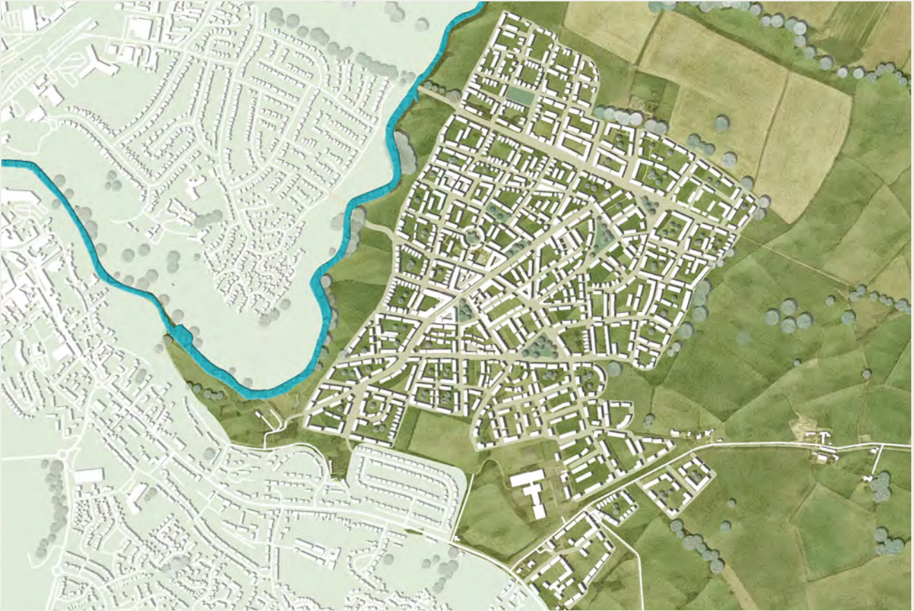
An alternative 'gentle density' masterplan using 230ha less land than the road-led masterplan
