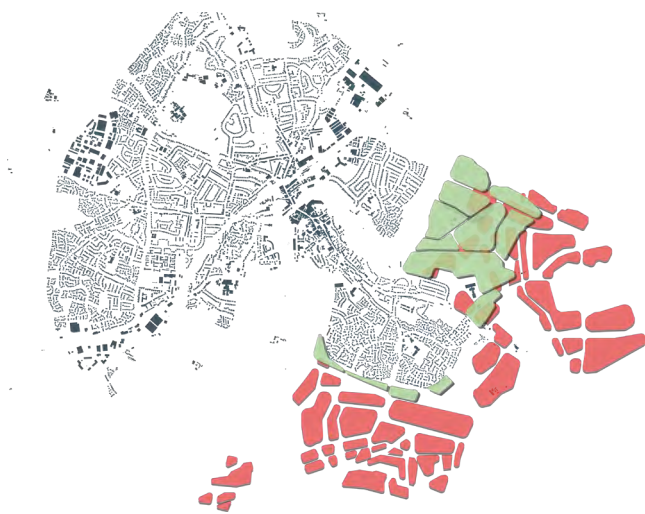
The vision-led masterplan (in green) showing significantly less land take than the road-led masterplan (in red)
